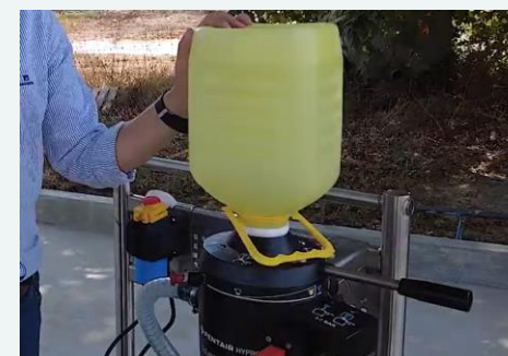
Figure 2: CTS with the container correctly sealed to the system
