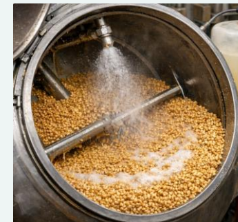
Figure 4: Seeds being treated with vinegar solution in seed dressing drum
