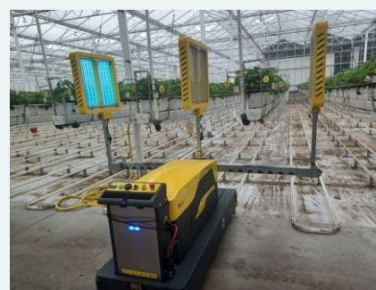
Figure 3: UV robot against powdery mildew in strawberry
