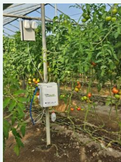
Figure 1: AcID Smart sensor system, the FILTER BOX can be spotted above the crops. Source: Project deliverables of AcID.
